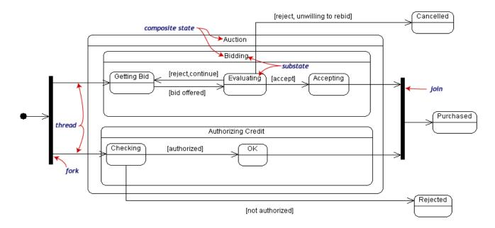
Entering the **Auction** requires a fork at the start into two separate threads. Unless there is an abnormal exit (**Cancelled** or **Rejected**), the exit from the **Auction** composite state occurs when both substates have exited.
