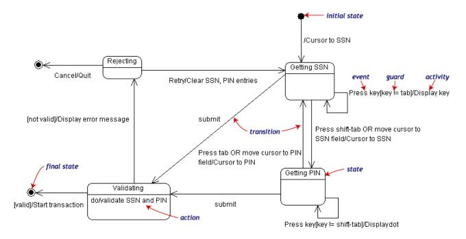
States are rounded rectangles. Transitions are arrows from one state to another. Events or conditions that trigger transitions are written beside the arrows. Our diagram has two self-transition, one on **Getting SSN** and another on **Getting PIN**.
