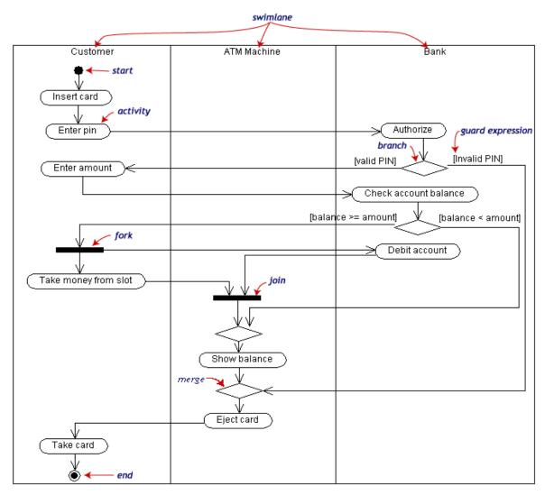
Activity diagrams can be divided into object **swimlanes** that determine which object is responsible for which activity. A single **transition** comes out of each activity, connecting it to the next activity.
