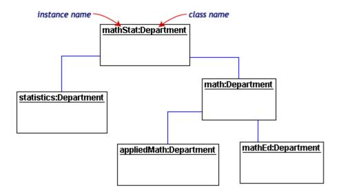
Each rectangle in the object diagram corresponds to a single instance. Instance names are underlined in UML diagrams. Class or instance names may be omitted from object diagrams as long as the diagram meaning is still clear.
