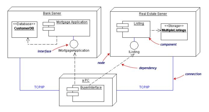
The physical hardware is made up of **nodes**. Each component belongs on a node. Components are shown as rectangles with two tabs at the upper left.
