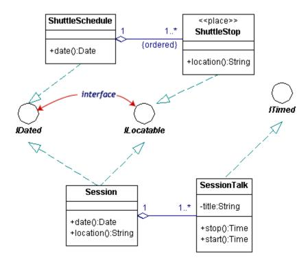
In circle notation, the interfaces are circles with lines connected to the implementing classes. Since it is more compact but leaves out some detail, the lollipop notation simplifies the original diagram.
