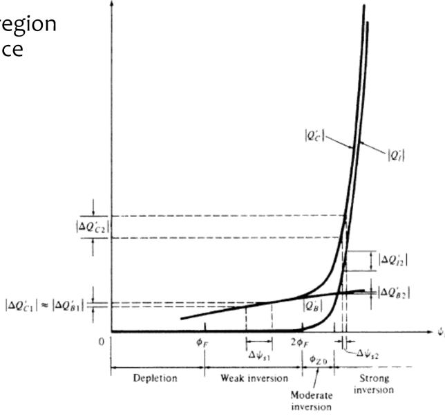
■Surface potential vs. gate-substrate voltage (right) and charges vs. surface potential (left).
