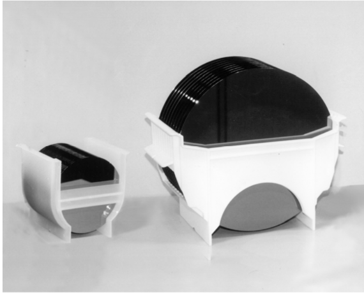
200-mm (8 in.) and 400-mm (16 in.) polished silicon wafers in cassettes. (Photo courtesy of Sin-Etsu Handotai Co., Tokyo.)
