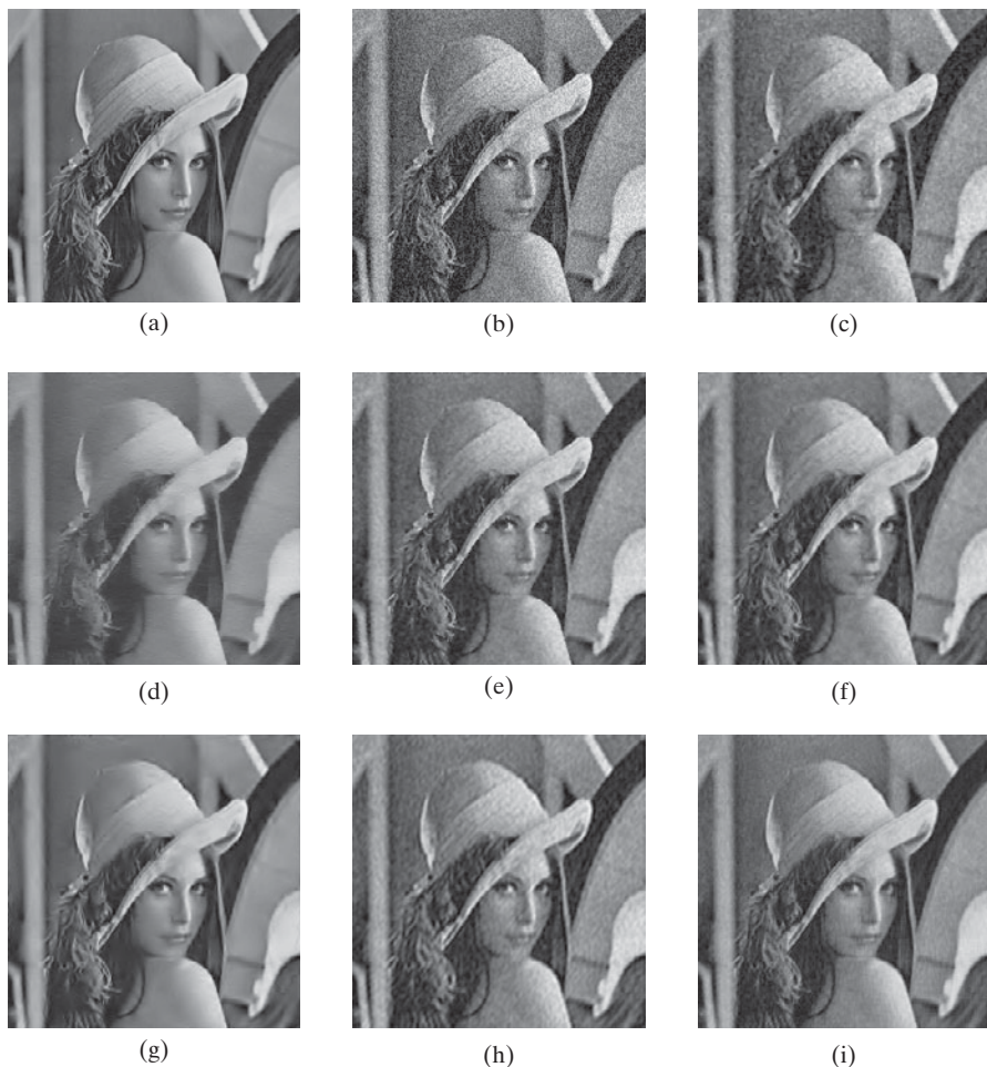
FIGURE 8.14 Denoising an image corrupted by white Gaussian noise: (a) Original image of Lena. (b) Input noisy image. (c) Median filter. (d) Matlab's wavelet denoising. (e) Matlab's Wiener filter. (f) Choi and Baraniuk's method. (g) Pižurica and Philips's method. (h) PCA ( r = 20 ). (i) KHA ( r = 40 ). (This figure is reproduced with the permission of Dr. K. I. Kim.)
