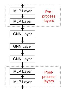
Pre-processing layers: Important when encoding node features is necessary.E.g., when nodes represent images/text
