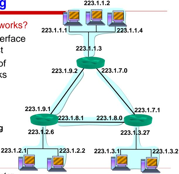
Interconnected system consisting of six networks.
