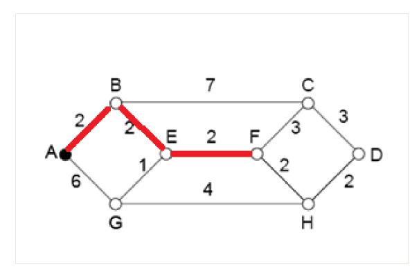
Shortest path from A to F using Dijkstra's algorithm
