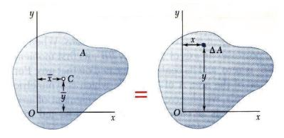
$$\bar{x} = \frac{\int x \, dW}{W} \quad \Rightarrow \quad \bar{x} = \frac{\int x \, (\gamma t) \, dA}{(\gamma A t)} \quad \Rightarrow \left( \bar{x} = \frac{\int x \, dA}{A} \right)$$
