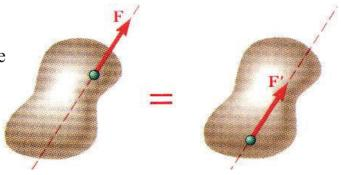
• Moving the point of application of the force **F** to the rear bumper does not affect the motion or the other forces acting on the truck.
