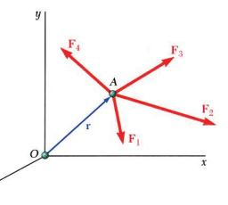
• Varigon's Theorem makes it possible to replace the direct determination of the moment of a force **F** by the moments of two or more component forces of **F**.
