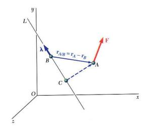
$$\begin{split} M_{CL} &= \vec{\lambda} \bullet (\vec{r}_{A/C} \times \vec{F}) = \vec{\lambda} \bullet [(\vec{r}_A - \vec{r}_C) \times \vec{F}] = \\ \vec{\lambda} \bullet [(\vec{r}_A - \vec{r}_B) \times \vec{F}] + \vec{\lambda} \bullet [(\vec{r}_B - \vec{r}_C) \times \vec{F}] \\ &\Rightarrow M_{CL} = M_{BL} \end{split}$$
