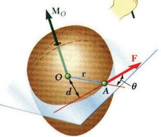
Any force F' that has the same magnitude and direction as F, is equivalent if it also has the same line of action and therefore, produces the same moment.
