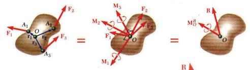
• The force-couple system at *O* may be moved to *O*' with the addition of the moment of *R* about *O*',
