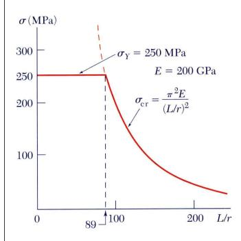
• The value of stress corresponding to the critical load,
