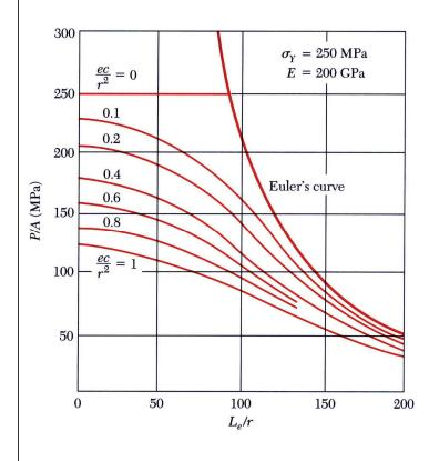
Load per unit area, P/A, causing *yield* in column
