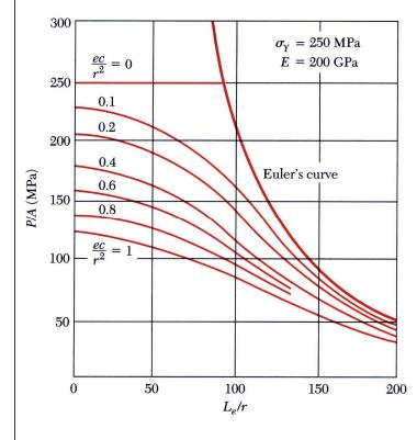
It should be noted that **for small values of KL/r**, the secant is almost equal to unity and P/A (or P) may be assumed equal to
