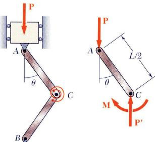
• Assume that a load *P* is applied. After a perturbation, the system settles to a new equilibrium configuration at a finite deflection angle.
