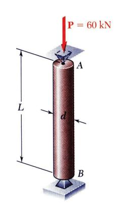
☐ Design of Columns Under Centric Load
