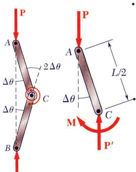
• Consider model with two rods and torsional spring. After a small perturbation,
