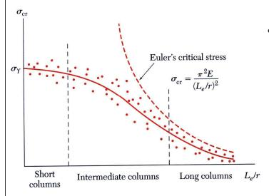
• Previous analyses assumed stresses below the proportional limit and initially straight, homogeneous columns
