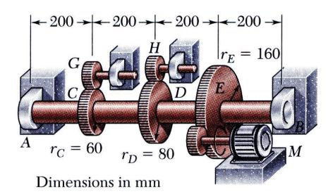
Solid shaft rotates at 480 rpm and transmits 30 kW from the motor to gears G and H; 20 kW is taken off at gear G and 10 kW at gear H. Knowing that  $s_{all} = 50$  MPa, determine the smallest permissible diameter for the shaft.
