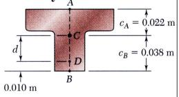
• Superpose stresses due to centric and bending loads
