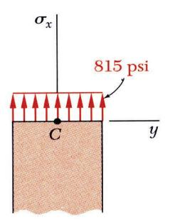
• Normal stress due to a centric load
