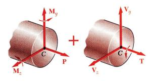
Axial force and in-plane couple vectors contribute to normal stress distribution in the section.
