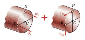
• Shear force components and twisting couple contribute to shearing stress distribution in the section.
