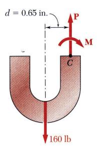
• Equivalent centric load and bending moment
