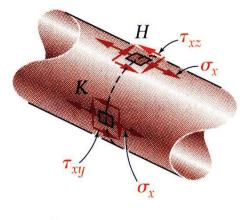
• Normal and shearing stresses are used to determine principal stresses, maximum shearing stress and orientation of principal planes.
