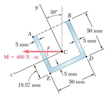
$$\begin{split} I_{y'} &= 281 \times 10^3 \text{ mm}^4 \\ I_{z'} &= 176.9 \times 10^3 \text{ mm}^4 \end{split}$$
