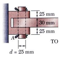
• To determine the bearing stress at A in the boom AB, we have t = 30 mm and d = 25 mm,
