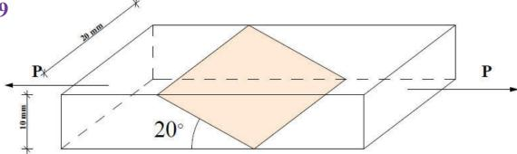
Two pieces of the wood beam are connected with glue connection. Determine the maximum safe axial load.
