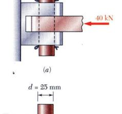
• The pin at A is in double shear with a total force equal to the force exerted by the boom AB,
