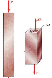
• The force intensity on that section is defined as the normal stress.
