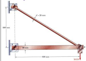
Can the structure safely support the 30 kN load? Assume that, the element CB has enough capacity.  $\sigma_{\text{all}_{AB}} = 165 \text{ MPa}$
