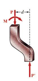
• If a two-force member is *eccentrically loaded*, then the resultant of the stress distribution in a section must yield an axial force and a moment.
