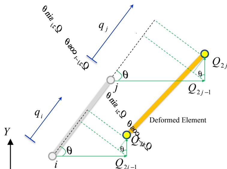
$$\begin{aligned} q_i &= Q_{2i-1} \cos \theta + Q_{2i} \sin \theta \\ q_j &= Q_{2j-1} \cos \theta + Q_{2j} \sin \theta \end{aligned} \quad (3)$$
