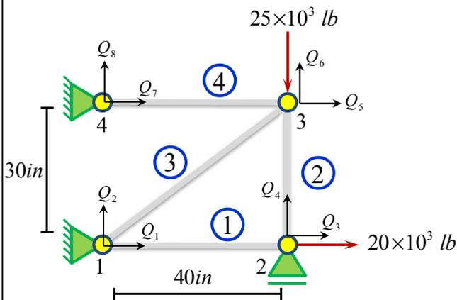
$$\sigma^{(3)} = \frac{29.5 \times 10^6}{50} \begin{Bmatrix} -0.8 & -0.6 & 0.8 & 0.6 \end{Bmatrix} \begin{Bmatrix} 0 \\ 0 \\ 5.65 \times 10^{-3} \\ -22.25 \times 10^{-3} \end{Bmatrix} \Rightarrow \sigma^{(3)} = -5208 \text{ psi} \quad (1.18)$$
