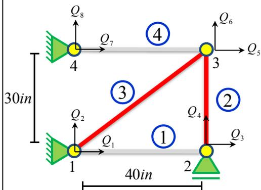
$$\sigma^{(3)} = 29.5 \times 10^6 \left( \frac{1}{50} \begin{Bmatrix} -0.8 & -0.6 & 0.8 & 0.6 \end{Bmatrix} \begin{Bmatrix} 0 \\ 0 \\ 0.003951 \\ 0.01222 \end{Bmatrix} - \frac{50}{150 \times 10^3} \right) \Rightarrow \sigma^{(3)} = -3643 \text{ psi} \quad (2.20)$$
