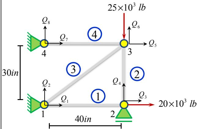
$$(20) \Rightarrow \sigma^{(e)} = \frac{E_e}{l_e} \begin{Bmatrix} -l & -m & l & m \end{Bmatrix} \begin{Bmatrix} Q_{2i-1} \\ Q_{2i} \\ Q_{2j-1} \\ Q_{2j} \end{Bmatrix}$$
