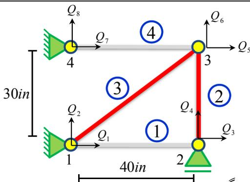
$$\begin{bmatrix} K_{11} & K_{12} & \cdots & K_{18} \\ K_{21} & K_{22} & \cdots & K_{28} \\ K_{41} & K_{42} & \cdots & K_{48} \\ K_{71} & K_{72} & \cdots & K_{78} \\ K_{81} & K_{82} & \cdots & K_{88} \end{bmatrix} = \frac{29.5 \times 10^6}{600} \begin{bmatrix} 22.68 & 5.76 & -15 & 0 & -7.68 & -5.76 & 0 & 0 \\ 5.76 & 4.32 & 0 & 0 & -5.76 & -4.32 & 0 & 0 \\ 0 & 0 & 0 & 20 & 0 & -20 & 0 & 0 \\ 0 & 0 & 0 & 0 & -15 & 0 & 15 & 0 \\ 0 & 0 & 0 & 0 & 0 & 0 & 0 & 0 \end{bmatrix} \quad (2.9)$$
