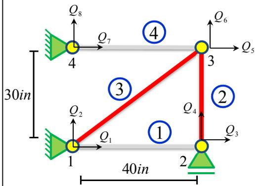
$$(28) \Rightarrow \sigma^e = E_e \left( \frac{1}{l_e} \begin{Bmatrix} -l & -m & l & m \end{Bmatrix} \begin{Bmatrix} Q_{2i-1} \\ Q_{2i} \\ Q_{2i-1} \\ Q_{2j} \end{Bmatrix} - \alpha \Delta T_e \right)$$
