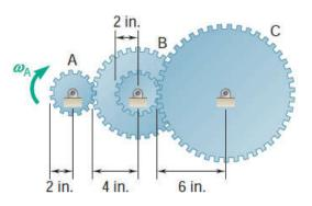
Key Answer: (a) 300 rpm 1, 100 rpm i. (b)  $a_B = 1974 \text{ in/s}^2 \text{ z}$ ,  $a_C = 658 \text{ in/s}^2 \text{ y}$ .
