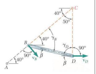
• Calculate the velocity at *D* based on its rotation about the instantaneous center of rotation.
