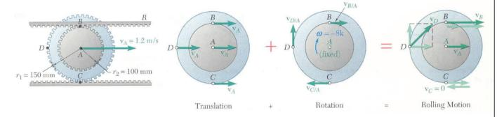
Velocity of the upper rack is equal to velocity of point *B*:
