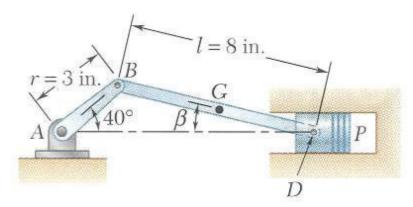
If the clockwise angular velocity of crankshaft AB is constant, which of the following statement is true?
