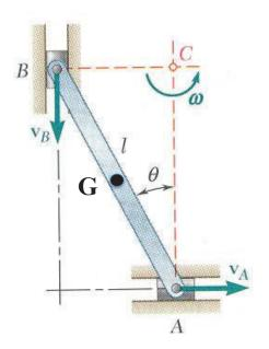
At the instant shown, what is the approximate direction of the velocity of point G, the center of bar AB?
