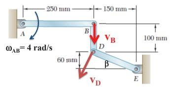
Locate instantaneous center C at intersection of lines drawn perpendicular to  $v_B$  and  $v_D$ .
