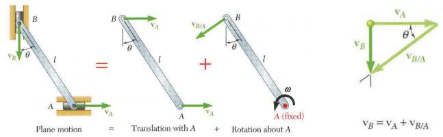
• The direction of  $v_B$  and  $v_{B/A}$  are known. Complete the velocity diagram.
