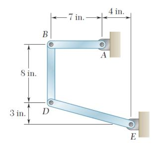
Knowing that at the instant shown bar *AB* has a constant angular velocity of 4 rad/s clockwise, determine the angular acceleration of bars *BD* and *DE*.
