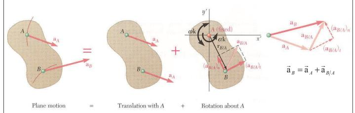
• Relative acceleration  $\vec{a}_{B/A}$  associated with rotation about A includes tangential and normal components,
