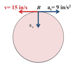
What is the direction of the normal acceleration of point *B*?
