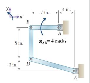
Determine  $v_{\scriptscriptstyle D}$  with respect to B.
