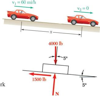
• Determine the distance required for the work to equal the kinetic energy change.
