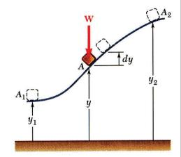
$V_g = Wy = potential energy$  of the body with respect to force of gravity.
