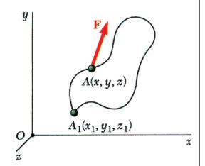
$$dU = -\left(\frac{\partial V}{\partial x}dx + \frac{\partial V}{\partial y}dy + \frac{\partial V}{\partial z}dz\right) \Rightarrow \vec{F} = -\left(\frac{\partial V}{\partial x} + \frac{\partial V}{\partial y} + \frac{\partial V}{\partial z}\right) = -\mathbf{grad}V$$
