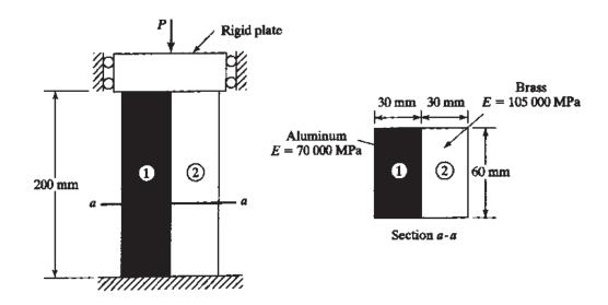
3.10. Consider the bar in Fig. P3.10. Determine the nodal displacements, element stresses, and support reactions.
