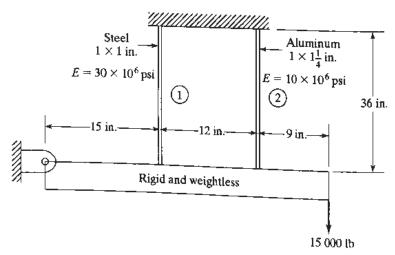
3.23. The structure in Fig. P3.23 is subjected to an increase in temperature,  $\Delta T = 80^{\circ}$ C. Determine the displacements, stresses, and support reactions. Solve this problem by hand calculation, using the elimination method for handling boundary conditions.
