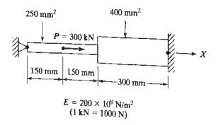
3.9. An axial load P = 385 kN is applied to the composite block shown in Fig. P3.9. Determine the stress in each material. (*Hint*: You may name the nodes 1-2 for both the elements.)
